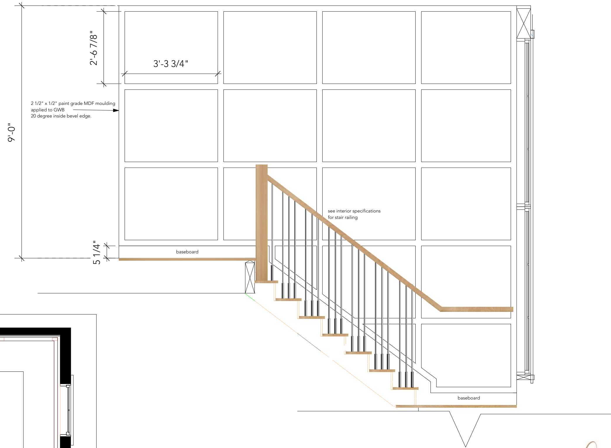
SECOND FLOOR STAIR WALL ELEVATION SCALE: 1/2"=1'-0"
